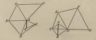
of gradually increasing the lengths of the sides away from a measured base AB; the second method is the better one.
